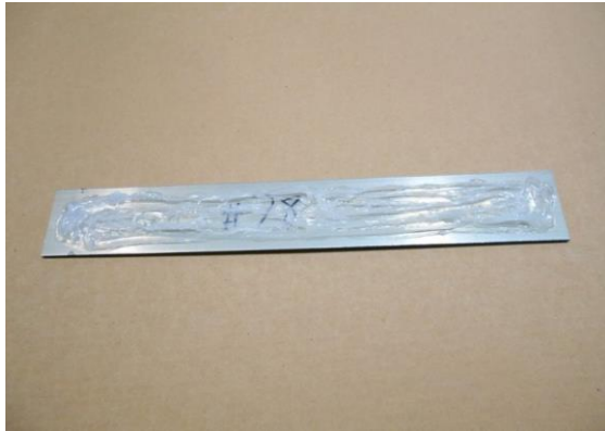
Figure 10 Caulk back of stop
